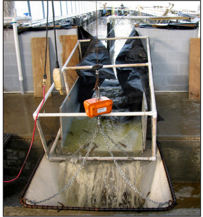
Figure 3. A concrete tank with a reinforced polyethylene liner. Wooden slats are removed from a portion of the end wall to quickly harvest shrimp into a net. Water is diverted to a temporary storage area and the net is hoisted up and rolled along an I-beam to a shrimp sorting station.
